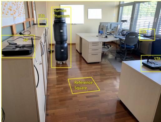
Fig. 3: Deployed testbed in an office environment.
