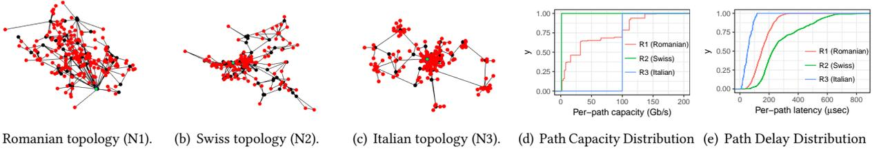
**Figure 4:** (a)-(c): Networks from 3 European operators: red dots indicate the BSS' locations, black dots the routers/switches, and the green dot an edge CU (placed at the most central position). (d)-(e) Path capacity and delay distribution for the 3 networks.
