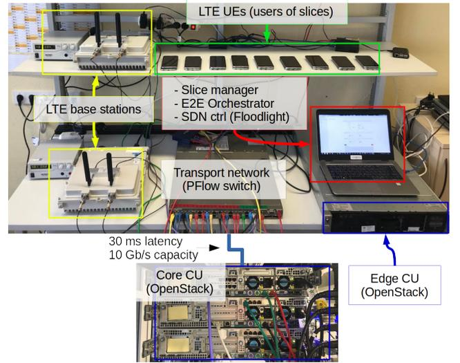
**Figure 7: Testbed**
